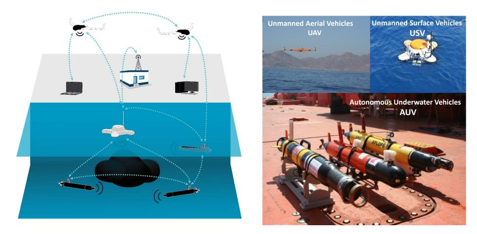
The multivehicle approach allows the use of relatively low-cost standard acoustic communications and oil in-water sensors, with novel advanced algorithms to get the most out these devices. The distributed intelligence of the networked devices across the spill is able to reveal a highly accurate and dynamic image of the spill. Ultimately, this cooperative multivehicle robotic technology allows a cheap, flexible, expandable, precise and rapid decision support system against oil spills.
