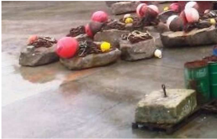
Fig. 11 Granite 3 tonne blocks chain and pick up buoys formed the oil boom's mooring, FHC.
