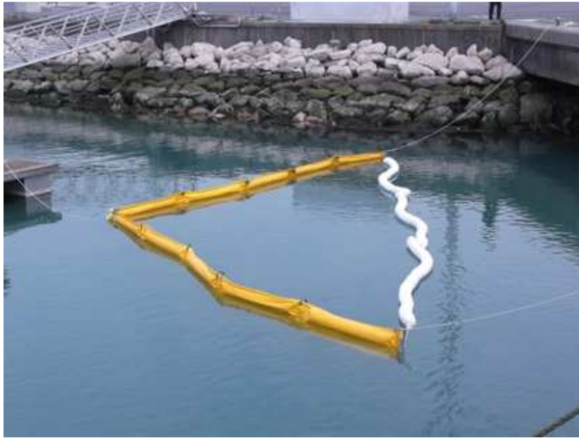
Fig. 18 Triangular sorbent and containment boom La Rochelle fishing harbour March 2015, EIGSI.
