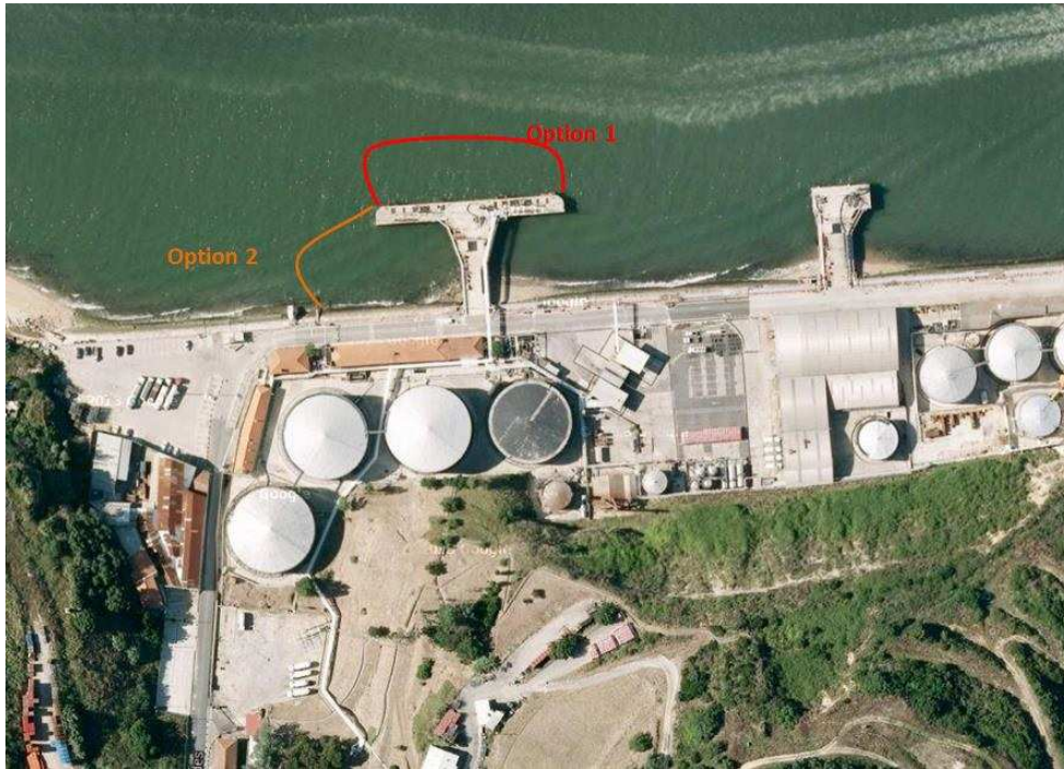
Fig. 13 Possible positions of the boom around the Banática liquid terminal at REPSOL terminal, Lisbon harbour experimentation, IST.
